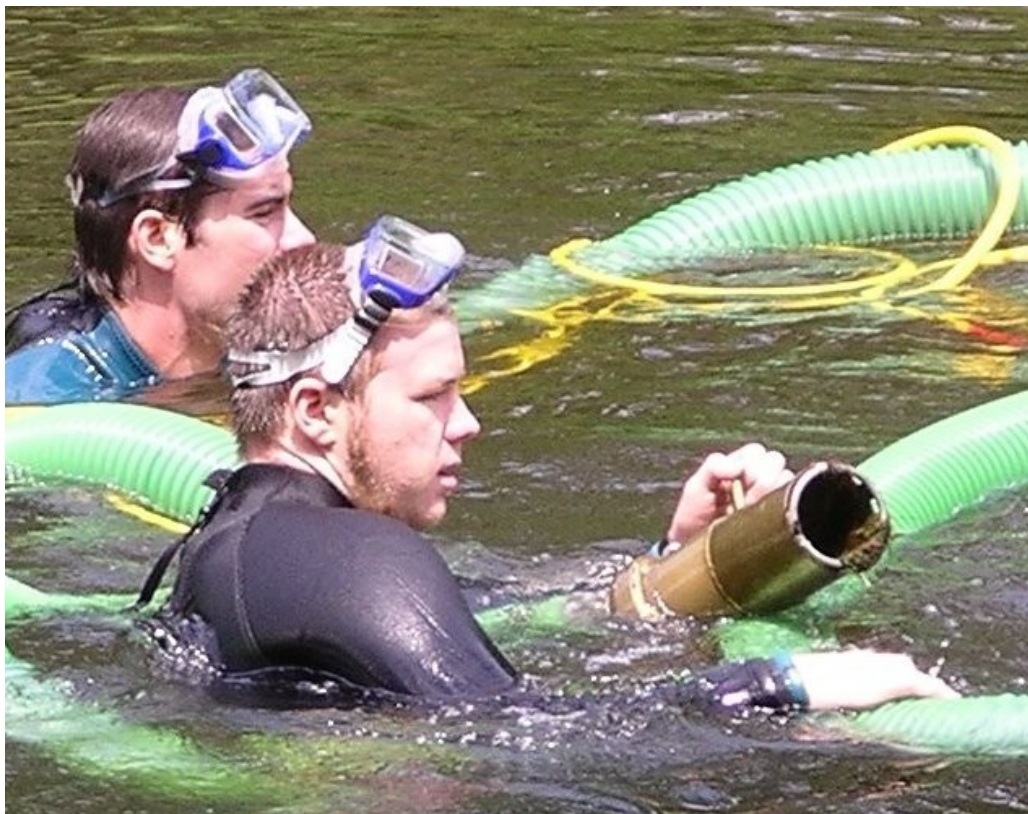
Figure 2- The working end of a DASH boat is rather like a vacuum cleaner, but it stays above the lake bottom to avoid disturbance of sediment and bottom habitat. A diver places an entire plant up into its intake nozzle, and only then gently pulls the entire root system loose – and up it goes for dewatering, bagging and removal.
