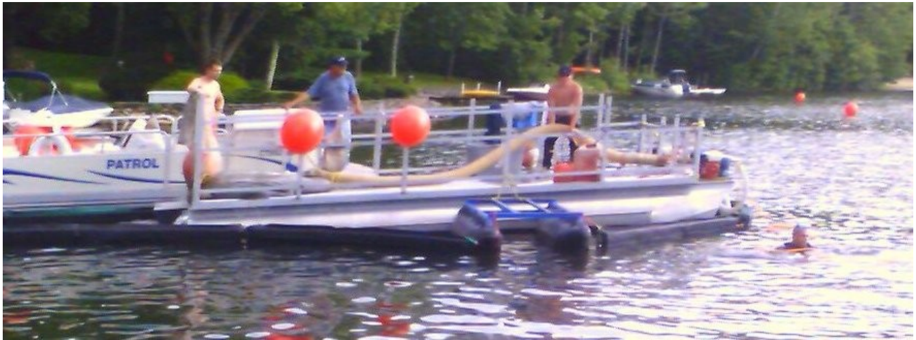
Figure 1- A UWS Aquacleaner DASH boat. Note orange hose on deck, and very large deck area for dewatering the harvested weeds. Black float tubes suspend a silt screen six feet into the water, to reduce lake turbidity from the draining operation; a black “gate” (with blue top rack) permits divers to enter and exit the screened area.
